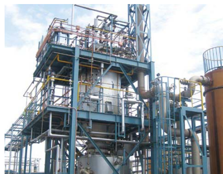
Submerged combustion-type waste liquid incinerator (Befu Works)
